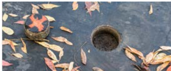
Figure 7: Remove the core from the hole
