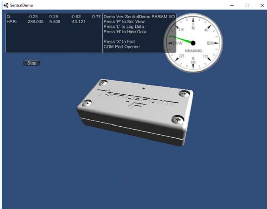
The data text box displays heading, pitch, and roll, in degrees, on the top line, and on the second line the quaternion values,  $Q_x$ ,  $Q_y$ ,  $Q_z$ , and  $Q_w$ . The compass dial provides real-time heading data in a common graphical format. The heading given on the compass dial matches the heading value in the data window.
