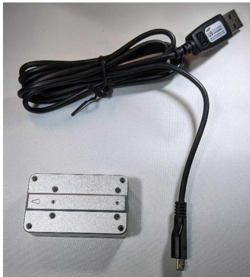
Figure 2 FORT Module with the arrow on the module and the micro USB cable
